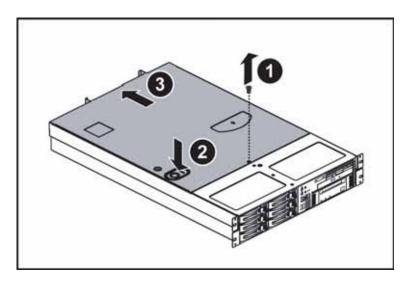
6 Slide the top cover (3) toward the back of the case, then lift it off the case.
